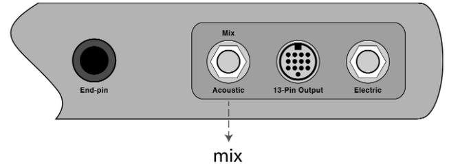
When an additional cable is inserted into output # 1 (electric output) the magnetic pickup signal is removed from the mix output so that there is now a separate output for both the magnetic and bridge transducer pickup systems.
